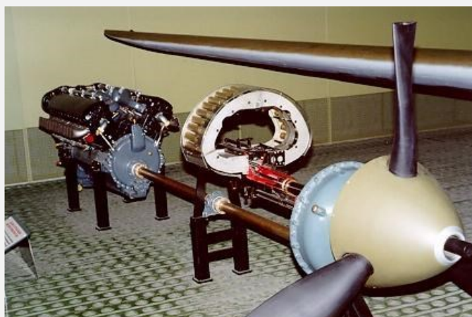
The T-9 cannon, produced by Oldsmobile, fired through the propeller hub.
